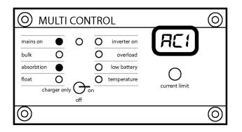
When the unit is plugged in and switched to "on" it is ready to use. The unit will switch over to battery power "Inverting" whenever power is lost. When power is restored the unit's charger will automatically recharge its batteries and continue to pass power through to the appliances it is supporting.
